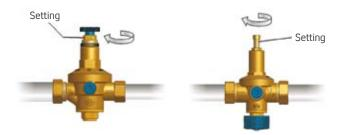
The outlet pressure (PS) is controlled by the rotating control or the regulation screw (according to the model); both present at the upper part of the device. The outlet pressure is increased by turning the rotating control clockwise, which is conform to current European legislation.
